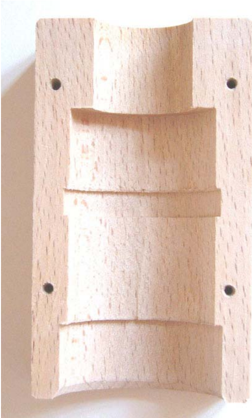
Correct! Sharp edges (no frays) Drilling correctly centered
