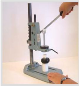
Place parts in the mounting machine
