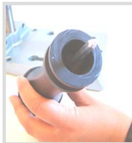
Check that the shaft is centered at the top
