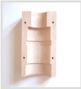
Make sure the drilling is correctly centered and with sharp edges (without burrs/frays)
