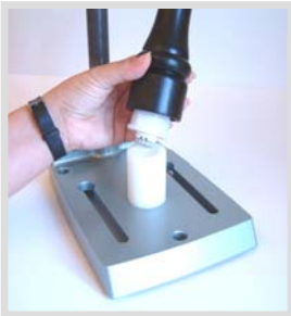
Place parts in mounting machine
