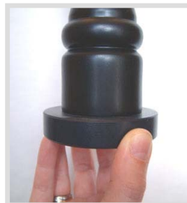
If products stands firmly (not wobbling) on the gauge then it has been mounted correctly
